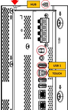
Use the short 10 cm USB cable supplied with the monitor. Connect USB cable from USB Type-B input marked with "Hub" (located above external speaker terminals) to USB Type-A input marked with "USB 1" on the side of the monitor. The red LED on the USB hub will light up.
