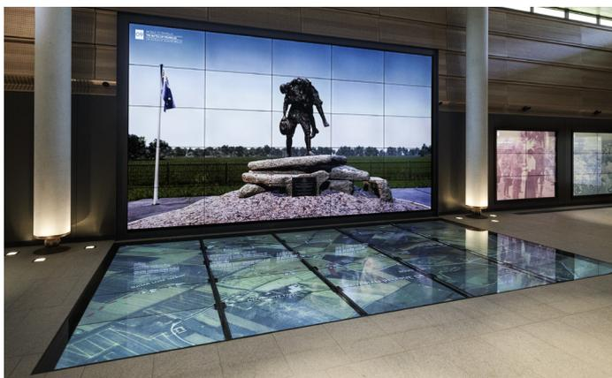
The final installation includes 50 55" X554UNS-2 ultra-narrow bezel displays (3.5 mm) ; 25 are deployed beneath a glass floor in front of the other 25 in a wall configuration.
