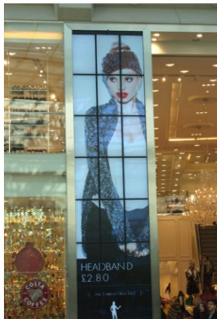
of the videowall. The sheer size and unique configuration of the project required extreme adaptability and presented a challenge in terms of installing and mounting the screens in a 3 x 7 portrait configuration. With no wall for attachment, the project required a bespoke mounting system which was custom designed and built by Unicol.
