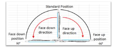
NOTE: Face-down installation is not supported by M431 PCAP, M491 PCAP, M551 PCAP & M651 PCAP .
