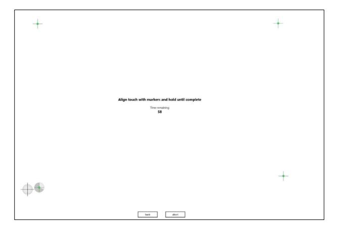
Note: It is normal for the green dots to not be aligned up with the cross hair shown on the circle, Dashboard will measure this offset and use it to calibrate the screen. Refer to the Application Note AN-FW-008 Calibration Process for detail instructions on how to calibrate the screen with the new GUI.
