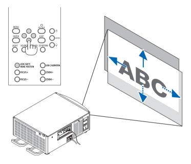
• Returning the lens shift position to the home position Press and hold the LENS SHIFT/HOME POSITION button for 2 seconds to return the lens shift position to the home position (nearly center position)
