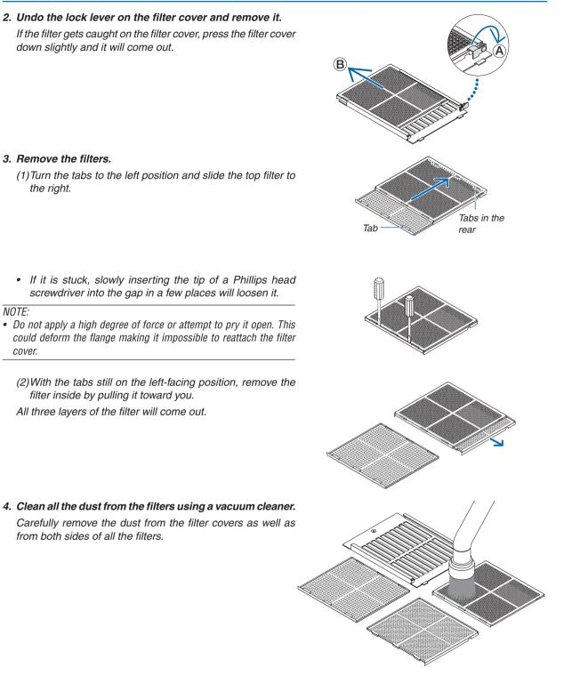
Remove the dust from the grates on the outside of the projector as well.
