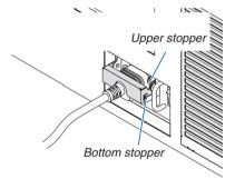
For releasing the fixing metal flap, pull it up until the fixing metal fits into the upper stopper.
