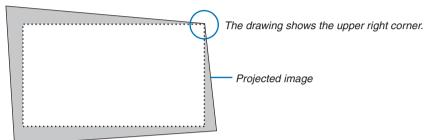
3. Pick up any one of the corners and align the corner of the image with a corner of the screen.
