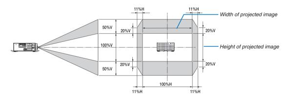
Description of symbols: V indicates vertical (height of the projected image), H indicates horizontal (width of the projected image).
