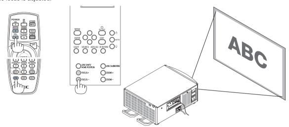
*TIP: To obtain the best focus, perform the following (for fixed installation) Preparation: Warm up the projector for one hour.*
