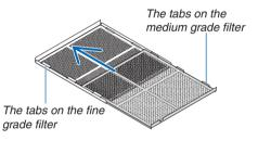
(2) Turn the tab slots on the coarse grade filter to the left. Next set the fine grade filter and the medium grade filter into the flange, then slide them to the left.
