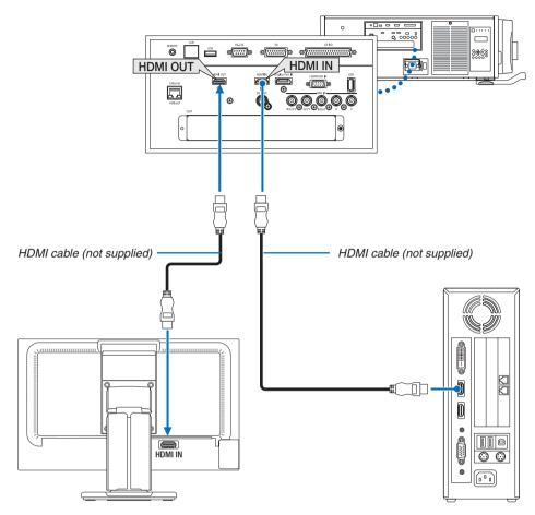
As shown in the figure, when the projector is connected to a computer, the same content from the HDMI input signal is displayed on the monitor for confirmation.
