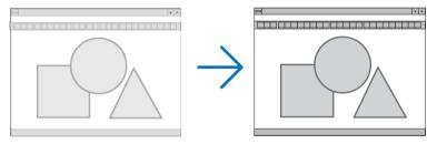
PHASE ...... Use this item to adjust the clock phase or to reduce video noise, dot interference or cross talk. (This is evident when part of your image appears to be shimmering.) Use [PHASE] only after the [CLOCK] is complete.
