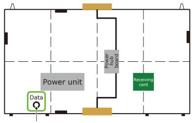
Hole for LAN cable connection
