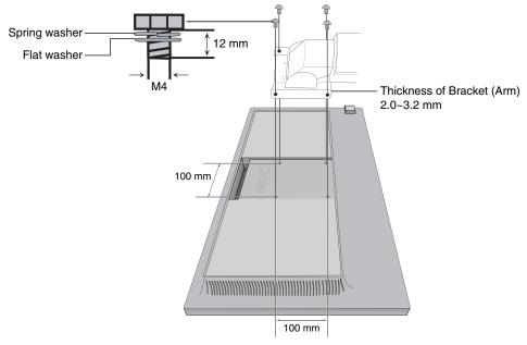
Weight of LCD assembly: 4.3 kg
