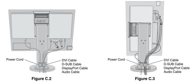
7. Connect one end of the power cord to the AC inlet on the back of the monitor and the other end to the power outlet.
