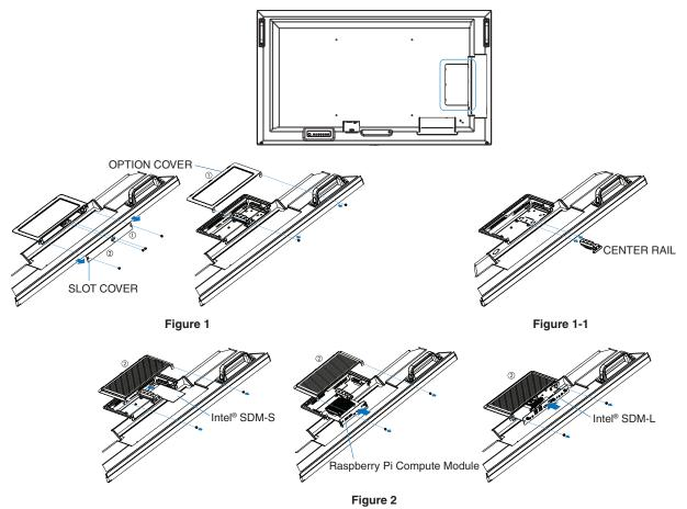
5. Insert the Option Board into the monitor and affix it in place with the removed screws (Figure 2). (Recommended fasten force: 50 - 80 N•cm).
