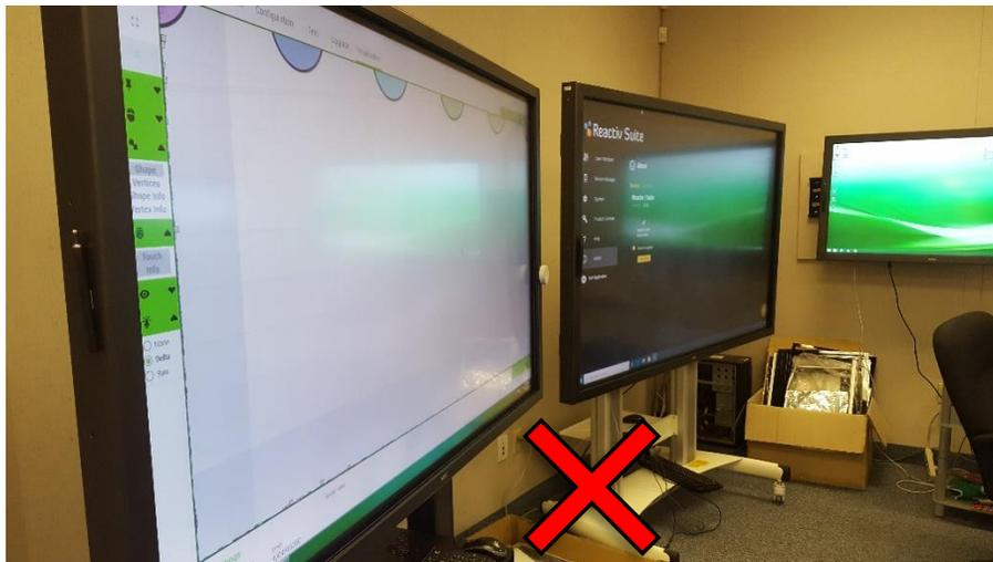
Notice there is a false shadow detection shown on the visualizer (left) that is being caused by the IR light bleed from the touch frame on the right:
